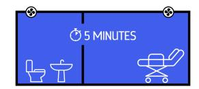
After 5 minutes of saturation, dry mist is evacuated and replaced with fresh air.
